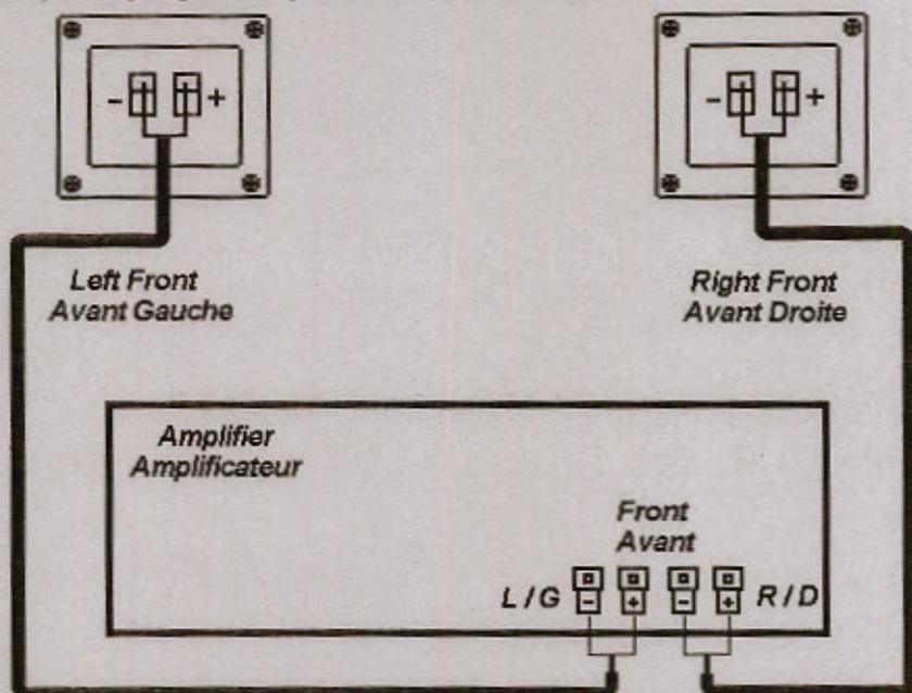
For normal operation of the M50 Ti, connect them to your amplifier's front channel output making sure that the positive (+) output from the amplifier is connected to the positive (+) input binding post on your speaker. Do the same with the negative (-) output and input.
